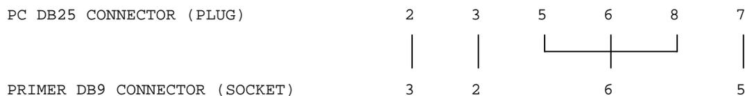
Some terminals require pins 2 and 3 of the DB25 go to pins 2 and 3 of the DB9 respectively:
